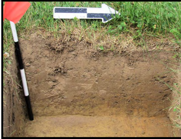
Figure 4: 50cm 2 shovel test pit. Note 20cm + A p overlying olive-yellow B/C horizon.
